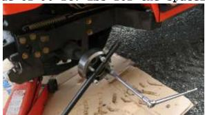
H. Get your socket & add Locktite to the studs on the spacer. Install the rim/wheel & now use the new nuts from the spacer, making sure they are flip to the proper end. Torque the nuts to 90 ft. lbs for the rim in the same 3 steps as above (3/4" Socket).
